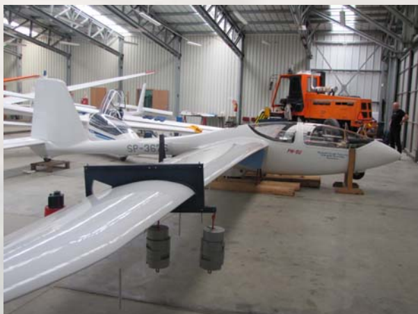
Figure 3: PW-6 glider during the verification wing stiffness tests
